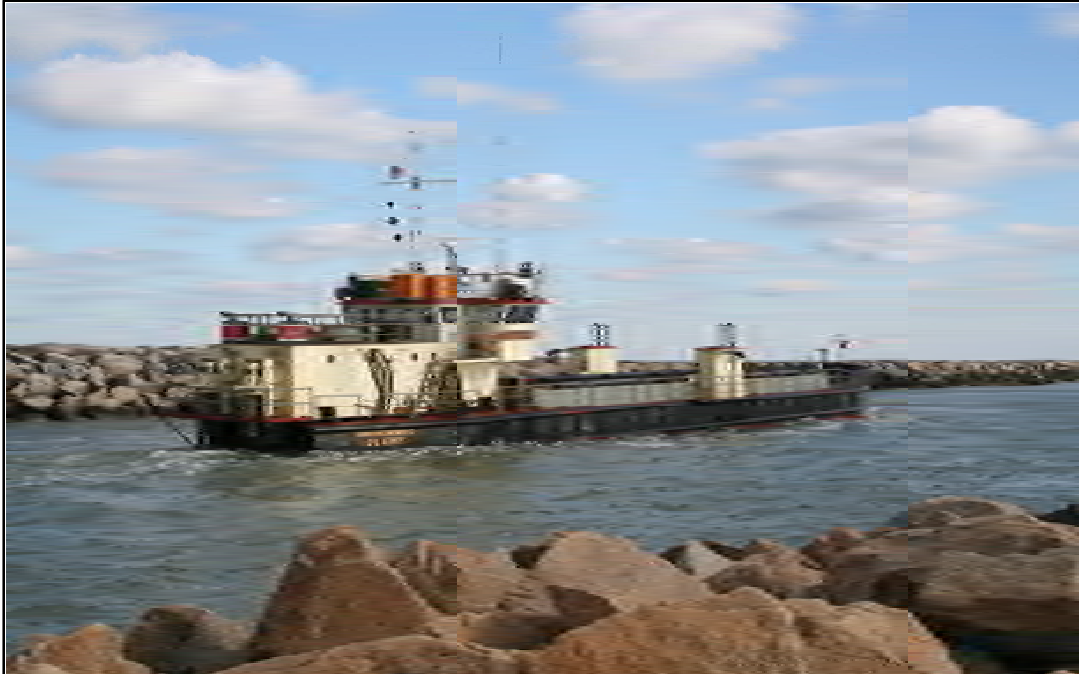
Figure 21 - The USACE Hopper Dredge Currituck. Cutter heads extend from the base of the dredge superstructure to agitate material on the seafloor. 28 June 2019.
