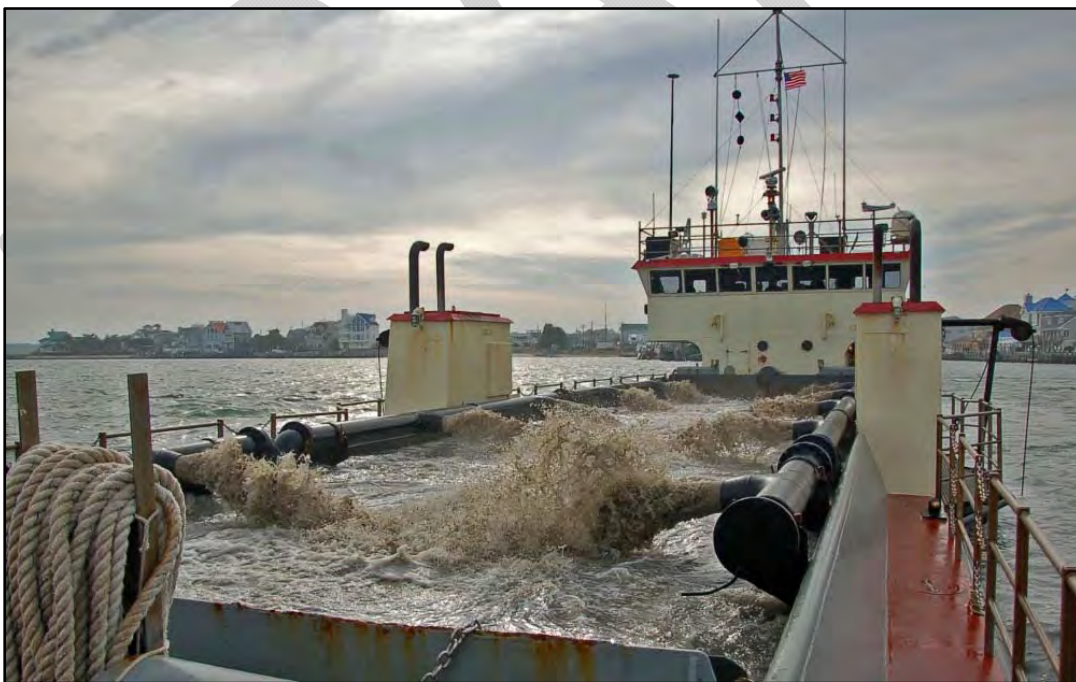
Figure 22 - USACE Hopper Dredge Currituck. Suction pumps draw a slurry of water and dredged sediment into the onboard holding cell. 28 June 2019.
