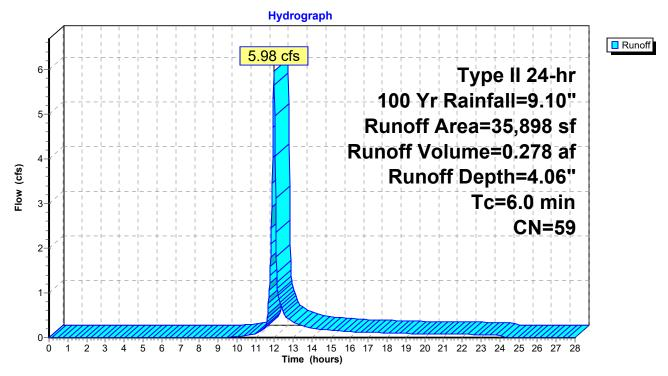
HydroCAD® 10.10-5a s/n 09480 © 2020 HydroCAD Software Solutions LLC
