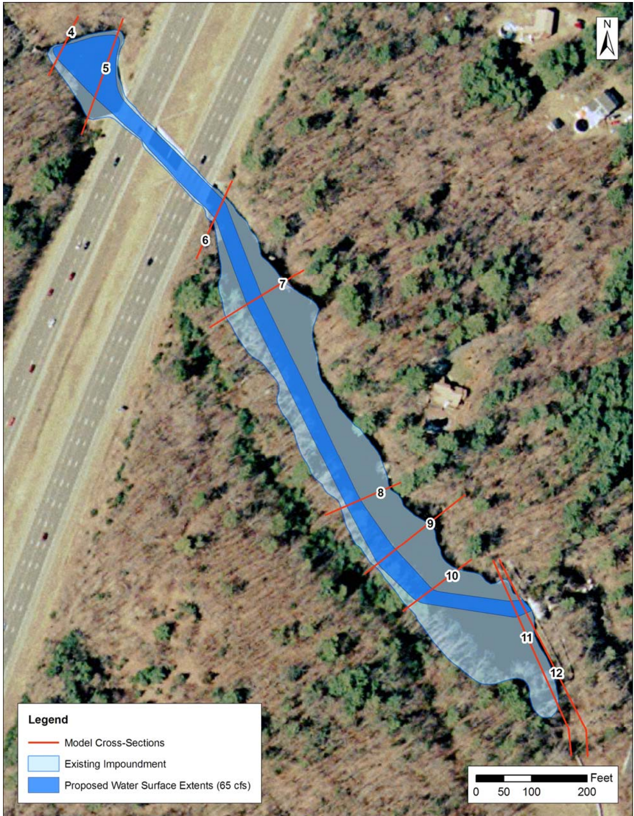
Figure E-5: Plan View of Larkin Road Dam Impoundment under Dam-in and Dam-out Conditions (Flow= 65 cfs)
